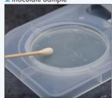
Inoculate the specimen on the center surface of the medium. A sterile inoculating loop that has been moistened by touching the surface of the medium may be used for inoculation of solids or scrapings.
