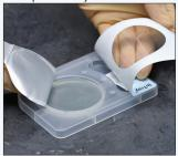
Allow tray(s) to warm to 18-25°C before use. Immediately label the tray with patient/sample information and date. Pull back the lower right corner adjacent to the clear window of the tray label until the protective seal is completely visible.
